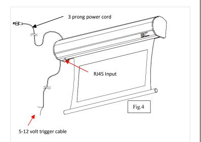
6. <u>Wireless 5-12 volt trigger</u> (Item F, Fig 5): The RF remote control serves as a dual purpose, independently as a handheld remote control, or in conjunction with the Wireless 5-12 volt trigger cable. The radio frequency technology can be programmed to send a wireless signal to synchronize its drop & rise with the projector's power cycle.
